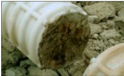
A successful grout test section
